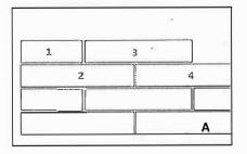
A. Products should be staggered in brick laid pattern, stagger equal to half of a plank for the first 2 rows, and then at least 18" for the following rows. Spacers should be placed against walls to maintain proper distance (3/8" to 1/2"). Tools needed: planks, underlayment, spacers
